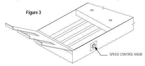
If the conveyor should fail to function, check for jammed paper between the tapes and roller. Also check the fuse and replace it if necessary. The fuse holder is located on the under side of the conveyor in the speed control box.
