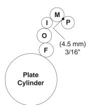
Turn the press on and run for 30-40 seconds to mill in the ink. Stop the press and allow it to sit still for 15-20 seconds. Jog the press forward and observe the stripe on the pan roller. It should be 3/16" (4.5mm). Turn the knurled metering knobs clockwise to increase the stripe and vice versa. When the proper stripe has been obtained, spin the rachet gears down until they bottom out on the stud and secure the rachet gear to the knurled knobs with set screws.
