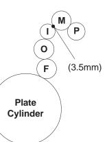
Replace the dampener metering roller and fully tighten the cap head bolt on the retaining bracket. Now you can ink up the entire dampener and run in the ink until it is smooth. The proper pressure between these rollers is 3.5 mm. Adjustments are made by loosening the lock nut on top of the metering roller hanger and turning the set screw clockwise to increase the stripe and vice-versa. Tighten the lock nut once the proper stripe is obtained.
