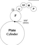
Shut the press off and drop the water form to the plate and back off again. (Form drops by moving single lever handle to water position). The form pressure to the plate should be set at 5/32". (Dropping the form to the plate leaves an ink stripe). Adjust the water form knobs (same ones used to adjust molleton form) until an even 5/32" stripe is achieved. Lock the position of the knobs with the small set screws. A stripe card is provided for your convenience.
