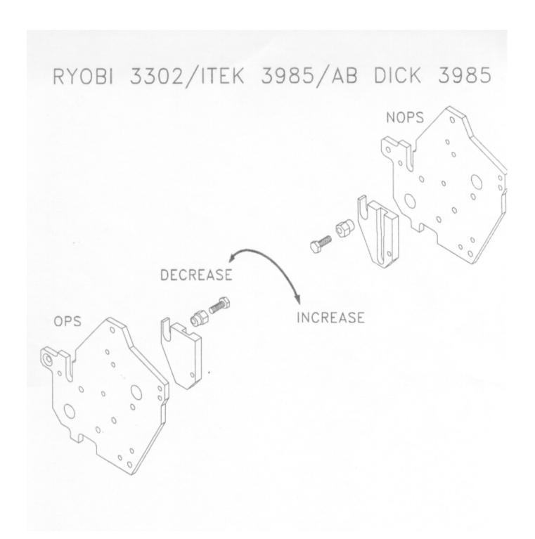
When adjusting the upper intermediate roll to the metering roll, turn the eccentrics in the direction indicated to set the stripe. The stripe between the intermediate and metering roll should be 1/8".
